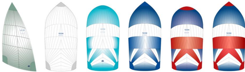
CODE ZERO LIGHT AIR REACHING S1 LIGHT AIR REACHING S2 LIGHT AIR RUNNING S3 MEDIUM AIR REACHING S4 MEDIUM/HEAVY RUNNING S5 HEAVY AIR SPINNAKER
